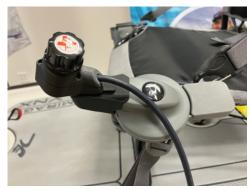
The motor deploys automatically only when the unit is in the water and the throttle is turned to the run position. The thrust from the propeller causes the motor to swing down and forward into position.
