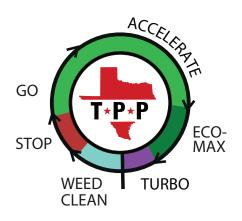
**ECO-MAX** - This region is the max speed for the proportional zone. To save battery life, the unit will sit in ECO-MAX unless put into TURBO boost.
